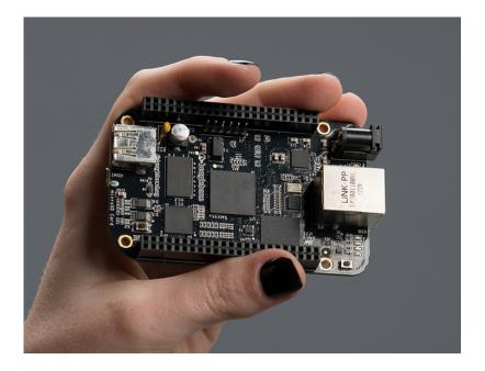
The BeagleBone Black includes a 2GB on-board eMMC flash memory chip. It comes with the Angstrom distribution factory pre-installed. You can flash new operating systems including Debian, Ubuntu, Android, and others. The following pages will illustrate the steps to getting the latest of each type of supported distribution onto the on-board eMMC.
