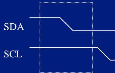
The first element we need to look at is the *Start* condition. A start condition indicates that a device would like to transfer data on the I<sup>2</sup>C bus.
