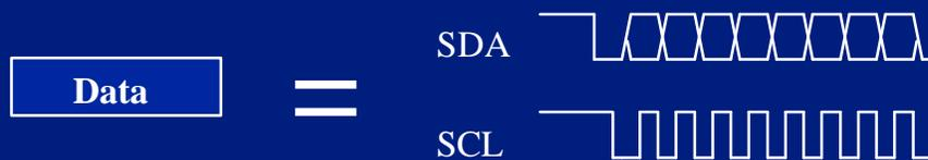
Let's now discuss the data transfer element. The data block represents the transfer of 8 bits of information. The data is sent on the SDA line and SCL produces a clock. The clock can be aligned with the data to indicate whether each bit is a "1" or a "0".
