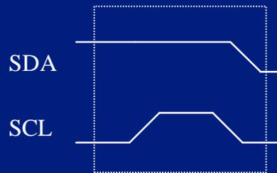
This is a *NACK* condition. Remember that a “ACK”s or “NACK”s a byte of data. I<sup>2</sup>C states that each byte **MUST** be answered with a NACK or ACK. If the device can not decide if it wants to ACK or NACK, then it will hold the clock line low until it makes up its mind. This action is known as “clock stretching” and is a feature of I<sup>2</sup>C to give devices enough time to respond. We will look at this in more detail later.
