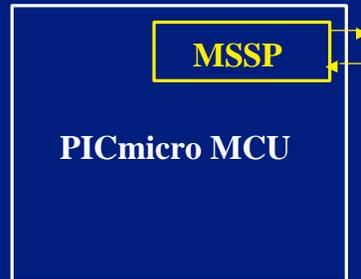
In the PICmicro, a module is used for the I<sup>2</sup>C protocol. This module is named the MSSP module and allows SPI or I<sup>2</sup>C to be implemented.
