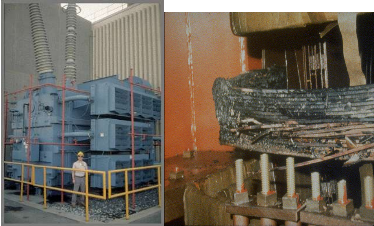
Figure 3. Generator step-up transformer owned by the Public Service Electric and Gas Company of New Jersey damaged by 13-14 March 1989 geomagnetic storm. Images provided courtesy of Public Service Electric and Gas and Peter Balma.
