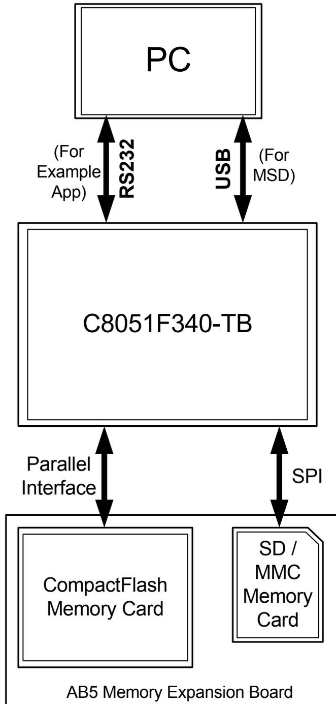
Figure 2. USB MSD RD Hardware Block Diagram
