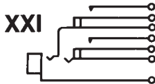
XXI Double open circuit. Isolated switching—separate “make” circuits on both tip and ring. (J2-2A).
