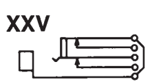
XXV Single closed circuit. Isolated switching “break” circuit. Sleeve common to isolated switching circuit throw. (J4-1B).
