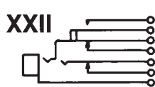
XXII Double closed circuit. Isolated switching “make” circuit on ring spring. (J7-1A).
