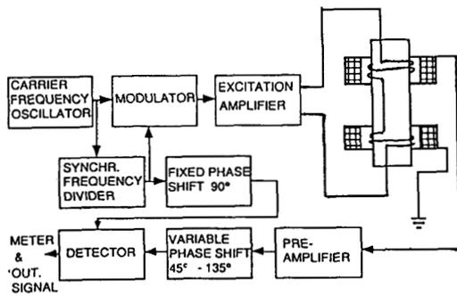
Fig. 2. Block diagram of the magnetometer.
