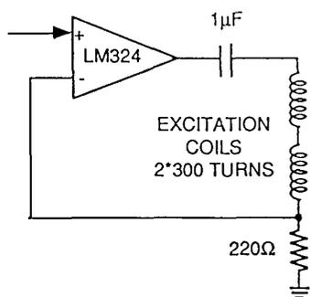
Fig. 4. The excitation system actually employed in the magnetometer.
