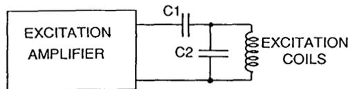
Fig. 3. The excitation system for the "trial and error" optimization procedure.
