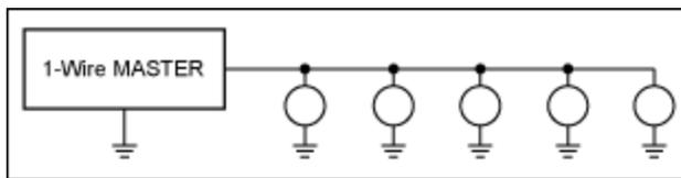
2. Stubbed topology. The 1-Wire bus is a single main line, starting at the master and extending to the farthest slave. Other slaves are attached to the main line through branches or stubs 3m or more in length.
