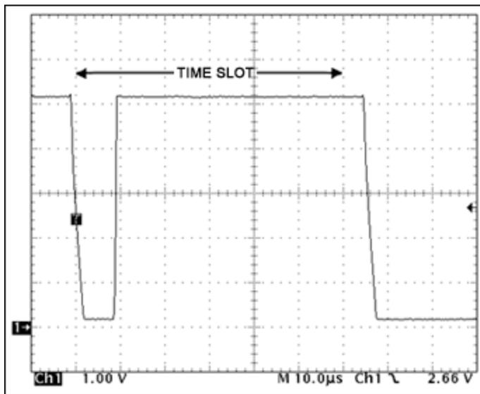
This image shows a Read One or Write One time slot. The master pulls the bus low for about 10µs and then releases it. Note the slow-rate-controlled fall time. The time slot lasts for about 70µs, after which another time slot occurs. Note that the time base is changed to 10µs per division.
