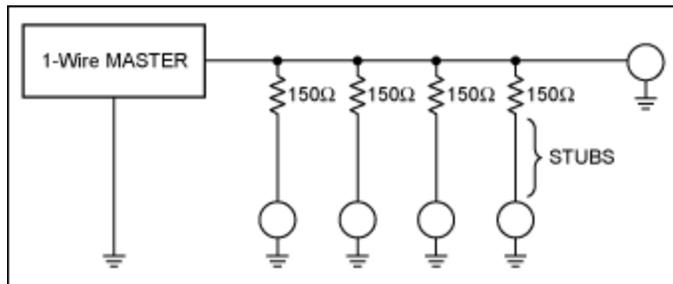
The most successful implementation of this concept uses 150Ω resistors at each point where a stub is connected to the main trunk. This value reduces the mismatch at the connection point by about 20%, and attenuates the resulting stub reflections by about 40%. However, the added resistance also degrades noise immunity by about 80%, so caution must be observed. Tests have also shown good performance using 100Ω resistor values, which do not degrade noise immunity quite as much.
