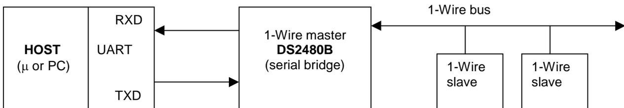
The minimum host UART that will work with this bridge must support 8-bit, non-parity, 9600 baud (bits per second) communication. Faster data rates up to 115200 baud can be negotiated but the bridge starts at 9600 baud when powering up. Electrical considerations such as RS232 are addressed in DS2480B data sheet.
